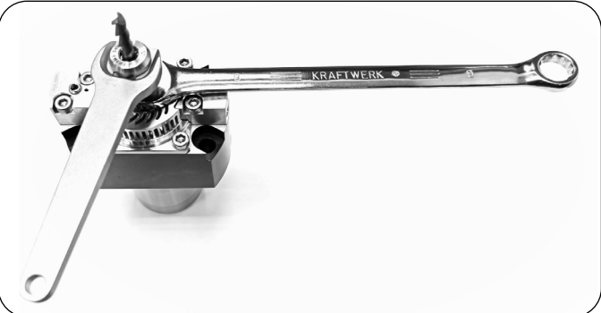
Fig. 3: Insert wrench into slots off the nut – turn counterclockwise
