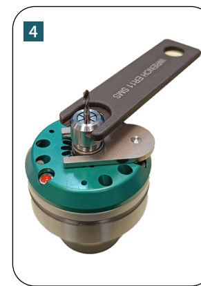
Fig. 5: Insert wrench into slots on nut – turn clockwise
