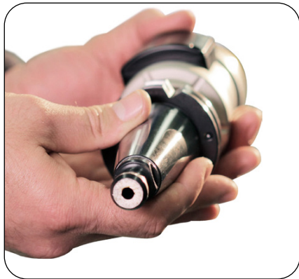
Fig. 20: Example of toolholder with a coolant-through hole
