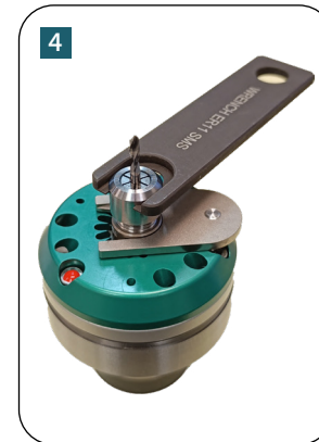
Fig. 25: Insert wrench into slots on nut – turn clockwise
