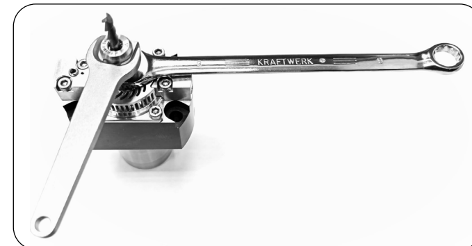
Fig. 9: Insert wrench into slots off the nut – turn counterclockwise
