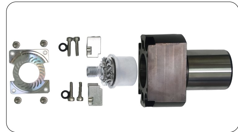
Fig. 14: SWISS JET Spindle taken apart for Cartridge replacement
