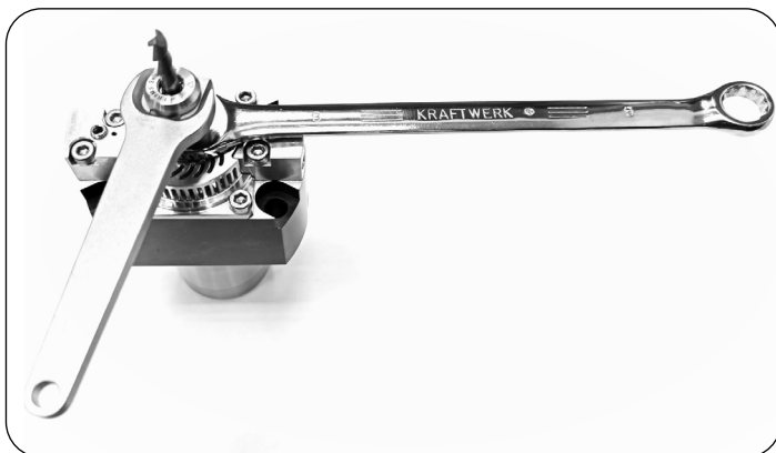
Fig. 5: SWISS Jet Spindle shaft lock mechanism
