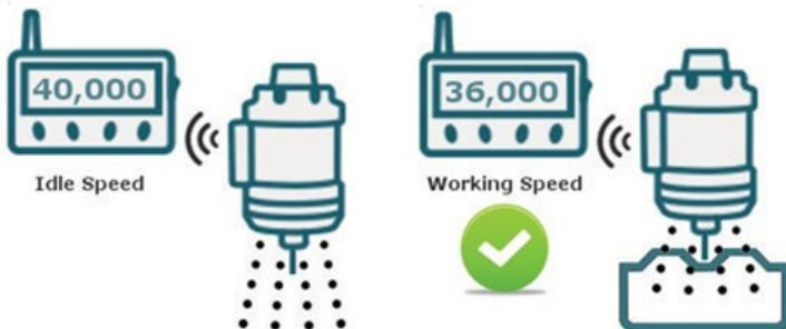
In the EXAMPLE, following the 10% rule: If idle speed is 40,000 RPM then during machining the jet spindle speed should decrease to a minimum of 36,000 RPM. If however, spindle speed decreases to less than 36,000 RPM, then both depth of cut ( $A_p$ ) and feed ( $F_z$ ) need to be reduced. Refer to Operating Data tables below.
