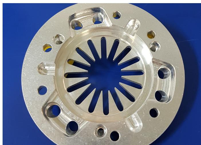
**HPC** Pocket, Slot & Plan Milling**HPC** Slot & Helical Milling
