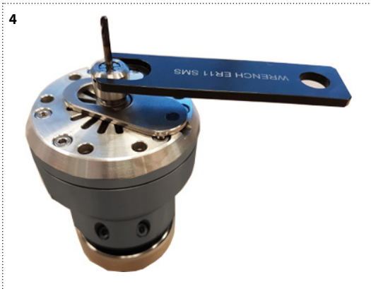
Fig. 35. Insert wrench into slots on nut – turn clockwise
