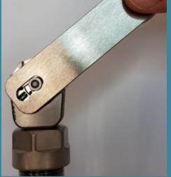
Insert Shaft Lock Wrench below Nut to stop spindle shaft from turning.
