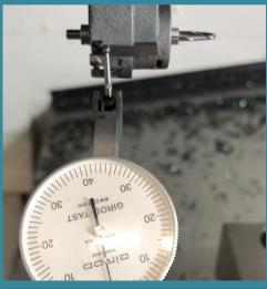
Use a dial to align on the grinded straight edge.
