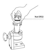
**3.C.** Set the ER32 built-in adaptor into the tool holder collet chuck and fasten the clamping nut.
