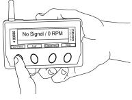
slide the transmitter across the left side of the display from point 1 to point 2.
