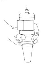
\* Don't forget to lock the main machine spindle during Jet Spindle operation.
