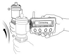
\*If side magnet does not make a connection, use magnets on the back of the display unit.
