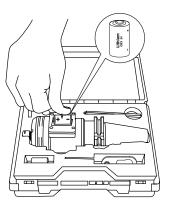
**1.C.** Replace screws to close the battery compartment.
