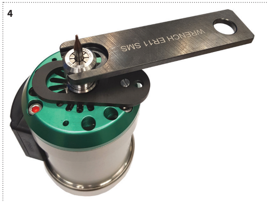
Fig. 35. Insert wrench into slots on nut – turn clockwise
