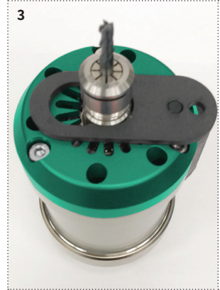
Fig. 34. Slide key into place
