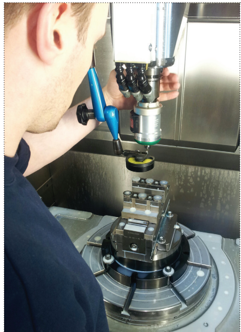
Fig. 37. Manual runout testing
