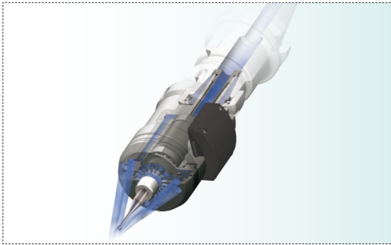
Fig. 10. Integrated coolant nozzle system
