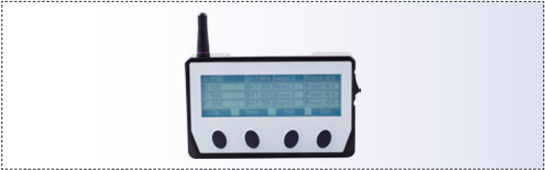
Fig. 18. List of connected HSM Jet Spindles on display
