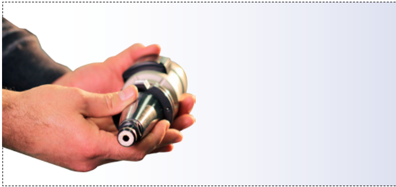
Fig. 30. Example of toolholder with a coolant-through hole
