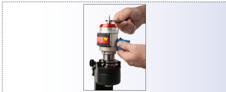
Fig. 36. Tightening ER11 nut
